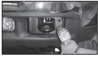
**1b.** On one side only, remove two bumper bolts on the front of bumper, out side of tow hook. These bolts will not be reused.
